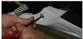
4. Remove catalyst cover. Remove O2 Sensor then catalyst.
