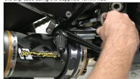
17. Check alignment and tighten muffler and the 4 6x14mm V.A.L.E.™ socket head cap screws.
