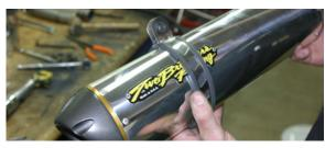
Slide the TBR muffler assembly onto the bike, and use the included spacer and bolt to loosely mount the canister to the bike as shown.
