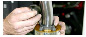
Slide the muffler clamp over the TBR S-bend, and slide the muffler canister clamp over the muffler canister.
