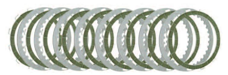
This kit does not include a diaphragm spring. Plates should be pre-soaked in the same fluid you will be using in the bike for about 10-15 minutes prior to installation. The type of fluids we recommend are Twin Power® Primary Lubricant (p/n 539018), or any HD petroleum based, non-synthetic, primary oil, as light weight as possible. *THE USE OF SYNTHETICS IS NOT RECOMMENDED AS THEY TEND TO CAUSE SLIPPAGE.*
