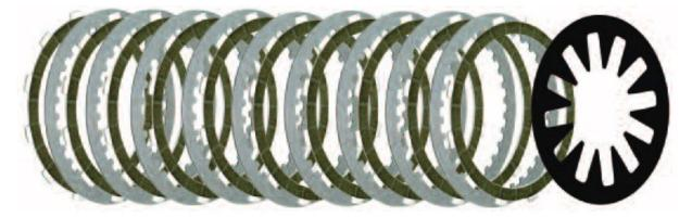
This kit includes a 10% stronger than stock diaphragm spring. Plates should be pre-soaked in the same fluid you will be using in the bike for about 10-15 minutes prior to installation. The type of fluids we recommend are Twin Power® Primary Lubricant (p/n 539018), or any HD petroleum based, non-synthetic, primary oil, as light weight as possible. <u>THE USE OF SYNTHETICS IS NOT</u> **RECOMMENDED AS THEY TEND TO CAUSE SLIPPAGE.**
