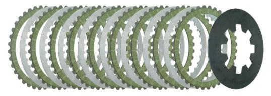
This kit includes a 15% stronger than stock diaphragm spring. Plates should be pre-soaked in the same fluid you will be using in the bike for about 10-15 minutes prior to installation. The type of fluids we recommend are Twin Power® Primary Lubricant (p/n 539018), or any HD petroleum based, non-synthetic, primary oil, as light weight as possible. <u>THE USE OF SYNTHETICS IS NOT</u> **RECOMMENDED AS THEY TEND TO CAUSE SLIPPAGE.**
