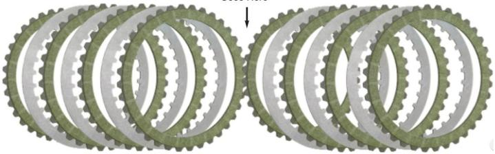
Plates should be pre-soaked in the same fluid you will be using in the bike for about 10-15 minutes prior to installation. The type of fluids we recommend are Twin Power® Primary Lubricant (p/n 539018), or any HD petroleum based, non-synthetic, primary oil, as light weight as possible. <u>THE USE OF</u> <u>SYNTHETICS IS NOT RECOMMENDED AS THEY TEND TO CAUSE SLIPPAGE.</u>
