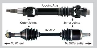
A "clunk" when accelerating, decelerating, or when putting the transaxle into drive. The noise comes from excessive play in either the inner or outer joints in a RWD independent suspension, or from the CV joints or U-joints in a RWD or 4WD powertrain. To verify the condition, back the vehicle up, alternating accelerating and decelerating, while in reverse. If the clunk or shudder is more pronounced, it confirms a bad joint.
