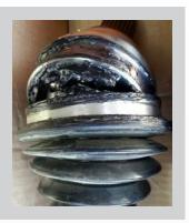
3. A humming or growling noise. This may be due to inadequate lubrication in either the inner or outer CV joint caused by a damaged or split boot. However, this symptom is more often due to worn or damaged wheel bearings, or worn shaft bearings.
