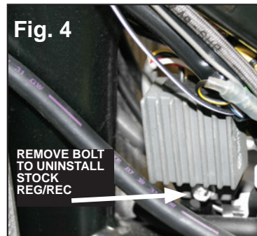
STOCK REGULATOR/RECTIFIER INSTALLED
