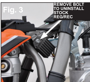
STOCK REGULATOR/RECTIFIER INSTALLED
