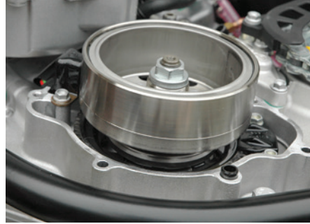
FLYWHEEL INSIDE ENGINE CASE
