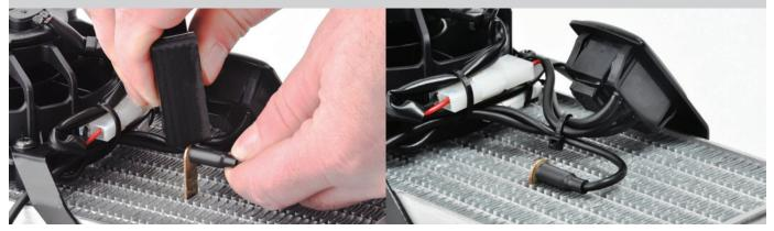
5.) Carefully insert the temperature probe into fins of radiator.
