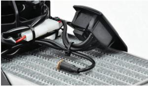
Carefully insert the temperature probe into fins of radiator.
