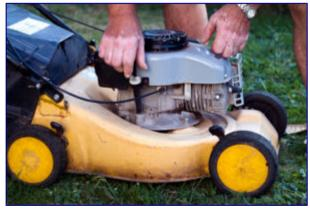
Make sure the engine is cool. Start by scraping off the built-up crust with a wire brush or putty knife. Then give the surface a good dose of SuperClean at full strength. We recommend SuperClean Aerosol Cleaner-Degreaser to get inside those nooks and crannies, and quickly break down the residual grass and mud. If necessary, gently brush the external surfaces, under the body, and the engine. Hose it off and you're on to the things you love to do in the summer heat! Super Easy. Super Fast.
