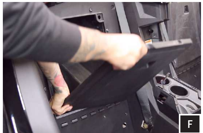
F. Remove pocket doors that cover both driver and passenger side.
