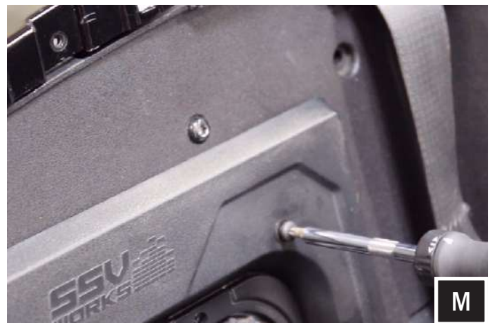
M. Attach the SSV Works logo plate using the T30 torx screws.
