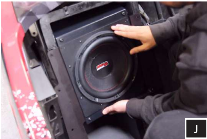
J. Grab the top and bottom of the enclosure and slide the sub box into place in the rear compartment
