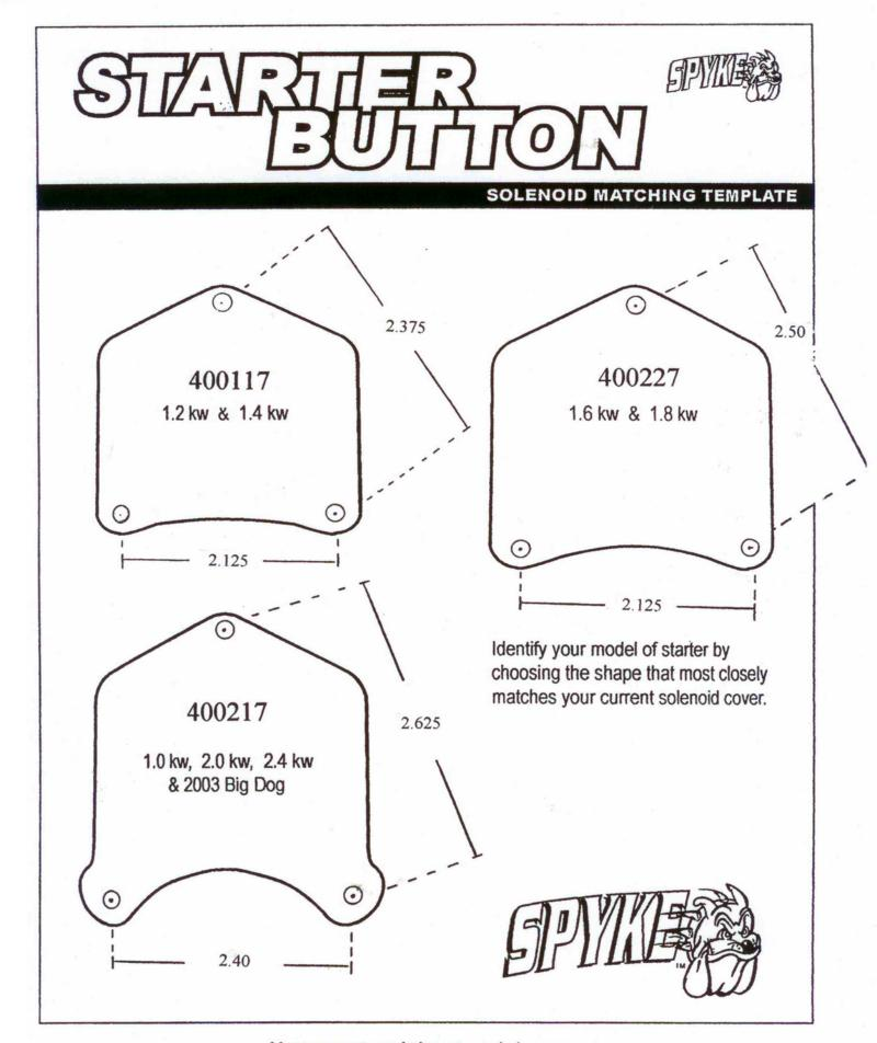
Measurements are hole center to hole center
