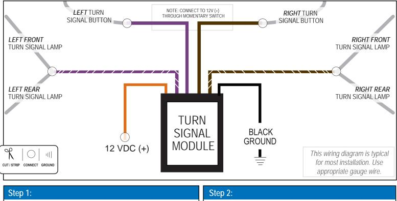
Follow wiring diagram by connecting all module wires to indicated wires above.
