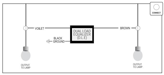
The Dual-Load Equalizer is designed to fix the problem when you have changed your stock directionals to L.E.D. turn signals and they flash quickly or not at all. It will equal the load that your system expects from the original incandescent bulbs by evening the load being sent and ultimately allow your signals to work properly.
