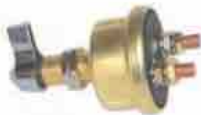
MP38910 LEVER OPERATED BATTERY DISCONNECT SWITCH Rated 175 A continuous, 800 A intermittent • 3/8" brass terminals • Chrome Plated Brass Lever • Includes faceplate
