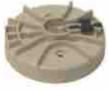
18-5245 ROTOR Replaces: 884790, 898253013 For: Late model V-6, V-8 (Alpha/ Bravo 350 Mag, 5.0L, & MX 6.2L)
