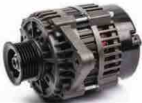
18-5984 ALTERNATOR Replaces: RA097007B 75/70 amp, spool mount, 2 5/8" OD, 6 groove serpentine pulley Clockwise position, 65mm
