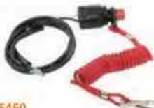
18-65450 EMERGENCY CUT-OFF SWITCH Replaces: Yamaha 6E9-82575-02-00 Push button kill feature Circuit closed with lanyard off. Use MP28860 replacement lanyard.
