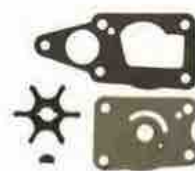
18-3266 WATER PUMP REPAIR KIT Replaces: 17400-98661 For: DF4, DF6 (2003-07)
