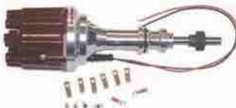
18-5481 HI-PERFORMANCE ELECTRONIC DISTRIBUTOR Fits: Ford V-8 351 Windsor Replacement cap/rotor kit: 18-5266
