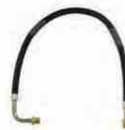
18-8115 FUEL LINE HOSE UNIVERSAL For fuel pump to carburetor connection. Replaces copper or steel tubing 3/8" X 25" PTFE composite hose with 5/8"-18 male inverted flare straight one end, 5/8"-18 90° one end. SAE J1527 type A1
