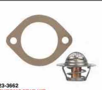
23-3662 THERMOSTAT KIT Replaces: Westerbeke 24688, 40434 Temperature Rating: 180° Fits: 20.0 SBEG(60Hz) / 16.0 SBEG(50Hz), 20.0 SBEGA(60Hz) / 16.0 SBEGA(50Hz), 22.5 SBEG(60Hz) / 18.7 SBEG(50Hz), 22.5 SBEGA(60Hz) / 18.7 SBEGA(50Hz)
