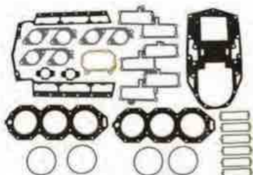
18-4428 POWERHEAD GASKET SET Replaces: 437725 Fits: 200 BB (1993 & Up), 225 BB (1993 & Up), 225 Ficht FFI (1999 & Up), 250 Carb only (2000)
