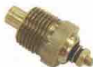
18-5898 SENDER Replaces: 97258A1, 97258, 34625, F16900198, F16900152 For Water Temperature 1/2" -14 NPT
