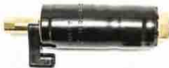
18-7326 ELECTRIC FUEL PUMP • 8 psi, 25 gpm Replaces: MerCruiser 805656A2, 805656A6, 805656A5, 805025A2, 861155A6, 861155A5 OMC/Volvo 3858261, 3850809, 3854620, 3857986
