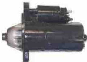
18-5920 STARTER Replaces: 987811, RK122014, RA122001 For: 5.0 & 5.8 litre Ford engines.
