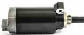
18-6438 STARTER Replaces: 50-888160T, 50-884045T, 50-859170T, 50-854636T, 50-893887T Fits: 30,40HP 3 Cyl 4 Stroke 0G760300 & UP
