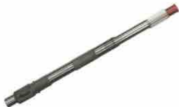
18-2187 PROP SHAFT Replaces: 395209 Cobra & Late Model 800 Drives
