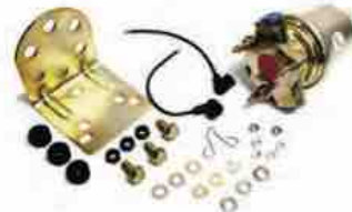
18-7333 ELECTRIC FUEL PUMP UNIVERSAL 12V, 72GPH at 5.75 PSI, 1/4" NPSF for 3/8" hose, for use with gasoline and diesel fuel. OPT72533 pressure safety switch recommended.
