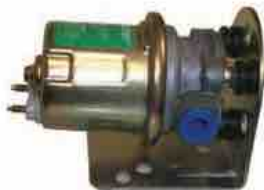
18-7332 ELECTRIC FUEL PUMP Includes bracket and mounting hardware 43 GPH - 7 PSI Max. - 1/4 NPSF for 3/8 hose - operates with both gasoline and diesel fuel - 24 Volt only
