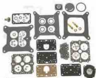
18-7096 CARB KIT Replaces: 982539, 85R-4541 (Contains adjustable needles and seats)
