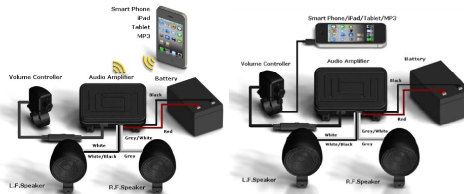
Figure 3. Wiring diagram for Waterproof Bluetooth Audio System. Please note that the wiring plan is the same for both Bluetooth and 3.5mm AUX users.
