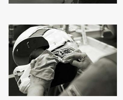
THE FINAL APPLICATION 7. Before a painted helmet shell is passed on for final assembly, the finished paintwork is given one last meticulous inspection. Perfection, even in areas that are unnoticeable by the untrained eye, is a must.
