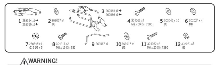
(B) Do not fully tighten the screws until it is ensured that the KIT is correctly attached and aligned.
