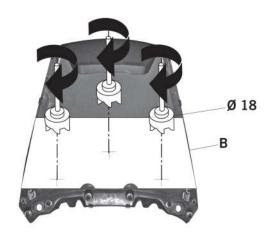
GB Place the stencil and make three 18 Ø holes (it is recommended to make an initial hole with an inferior diameter and progressively increase it). Assemble the back cover (B).
