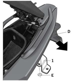
GB Disassemble the rear mudguard (D) by means of the nuts (E), assemble the reinforcement support (1) between the chasis and the rear mudguard (D) by means of the nuts (E).
