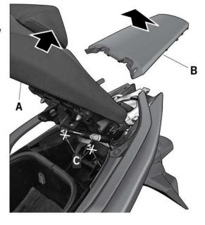
**(B)** Open the seat (A) and disassemble the back cover (B). Disassemble and discard the front screws (C) holding the seat's mechanism.
