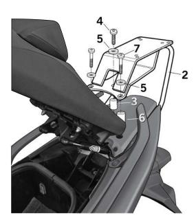
GB Assemble the KIT TOP support (2) in the upper central zone by means of the spacer (3), the screw (4) and the washer (5); and in the upper front zone by means of the spacers (6), the screws (7) and the washers (5).
