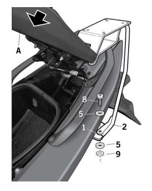
(B) Last, attach it to the reinforcement support (1) in the lower zone by means of the screws (8), the washers (5) and the nuts (9). Close the back seat (A).
