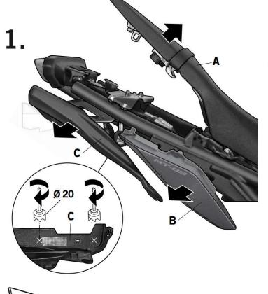
**GB** Open the seat (A). Disassemble the lateral covers (B). Disassemble the lateral fairing (C) and make two Ø20 mark holes on it. Assemble the lateral fairing (C) and the lateral covers (B).
