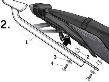
GB Assemble the KIT TOP support (1) by means of the spacers (2), the washers (3) and the screws (4). Close the seat (A).
