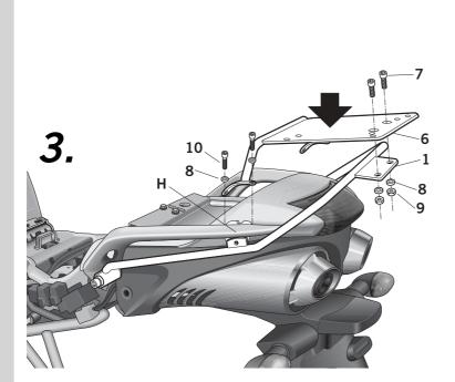
Then assemble the KIT TOP grill support (6) in zone (G), with the screws (7), washers (8) and nuts (9) and in zone (H), with the group of straps (4L-4R)(5L-5R), the screws (10) and washers (8).
