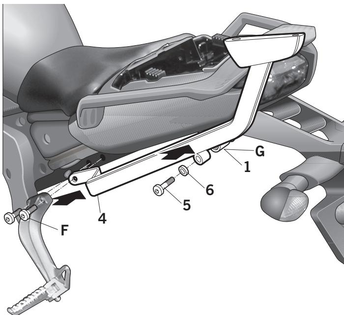
Dismount the back footrests with screws (F). Mount the KIT TOP support (4) with screws (F) between the motorbike's chassis and the footrests. And in zone (G), connect it to the connection support (1) with screws (5) and washers (6).
