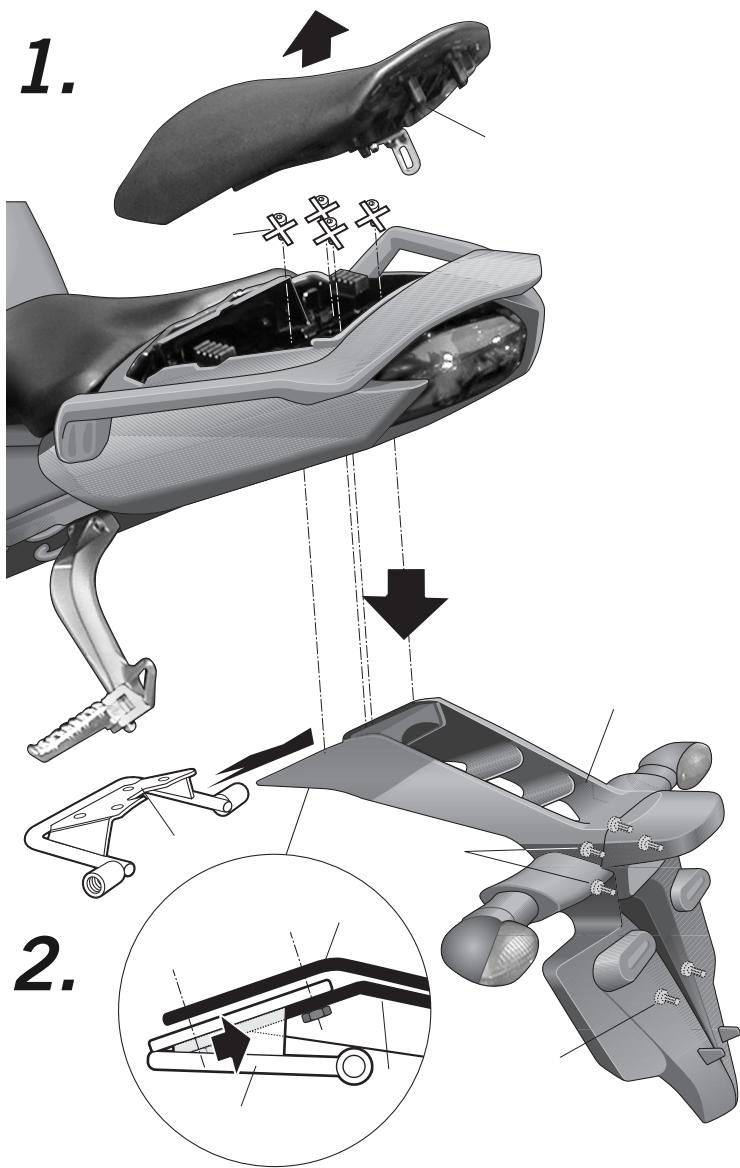
Dismount the back SEAT (A). Dismount the back mudguard (B), with screws (C) that will be eliminated.
