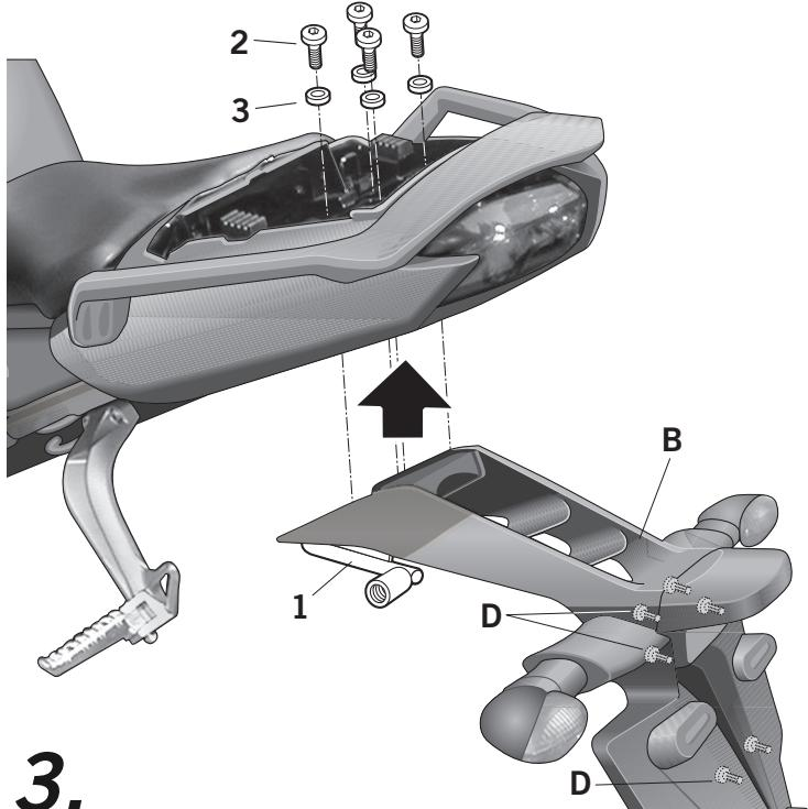
Loosen all the screws (D) that hold the reinforcement (E) plate of the back mudguard (B). Next, place the connection support (1) between the back mudguard (B) and its reinforcement (E) plate, according to the drawing.
