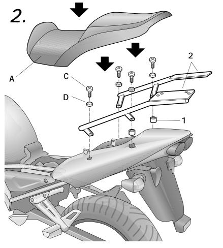
Position the spacers (1). Position the top kit supports (2), using the screws (C). Fit the seat (A).
