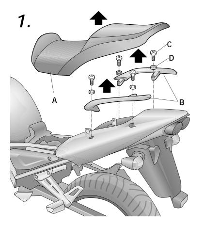
Advice for correct fitting of the kit: Do not fully tighten the screws until sure that the kit is correctly positioned and aligned.
