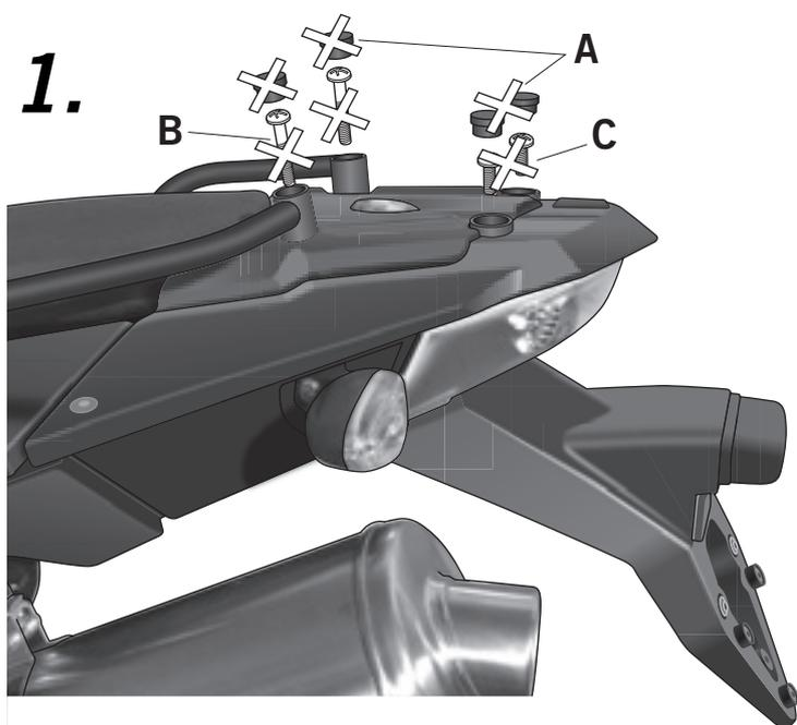
Disassemble and discard the motorcycle's handle caps (A). Disassemble and discard the screws (B) and the back screws (C).
