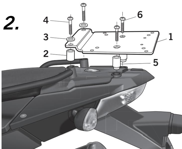
Assemble the KIT TOP support (1) in the front zone by means of the short spacers (2), washers (3) and screws (4) and in the rear zone by means of the long spacers (5) and the screws (6).
