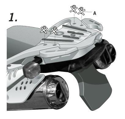
Remove and put aside the screws (A) of the original rear carrying case.
