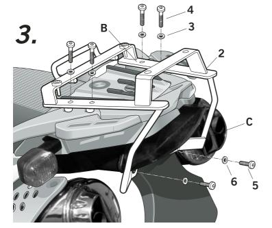
Next, assemble the Kit Top support (2) in area (B) using the spacers (1), washers (3), and screws (4). And in area (C) using the screws (5) and the washers
