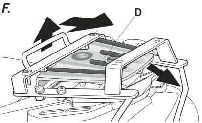
To be able to disassemble the cover of the rear carrying case (D) of the motorcycle, follow the steps as shown in our diagrams (E-F-G).
