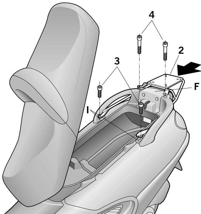
Assemble the KIT TOP (2) with the screws (3) in the zone (I), and screws (4) in the zone (F).
