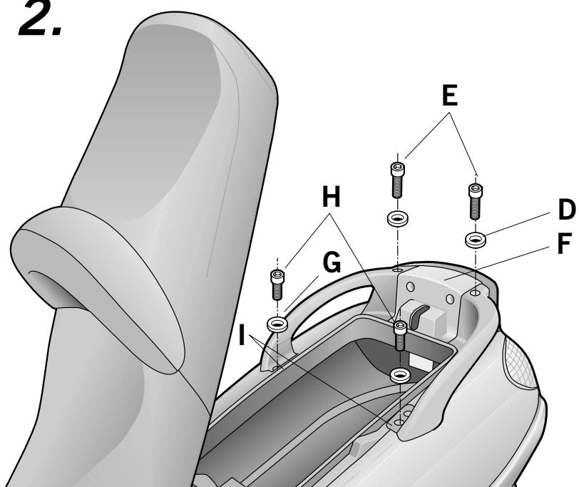
Loosen and remove the washers (D) and the screws (E) in the zone (F), and the washers (G) and the screws (H) in the zone (I).
