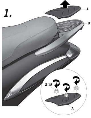
GB Disassemble the plastic embellisher (A). Make three Ø18 holes in the plastic embellisher (A) following the three marks found in the inferior part of the luggage rack (B). Once the three holes have been made, reassemble the plastic embellisher (A).
