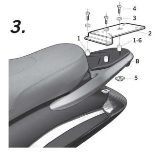
GB Place the cases (1) over the original luggage rack (B). Assemble the KIT TOP support (2) to the original luggage rack (B) by means of the cases (1), the washers (3), the screws(4) and the fixing plate M8 (5).
