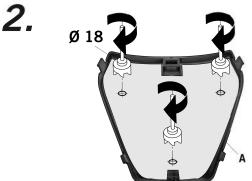
GB NOTE: For the Beverly sportouring 350/350i'12 model, a holes must be made over the plastic trim (A) using the template included in the instructions, and the spacer (6) in posterior area.
