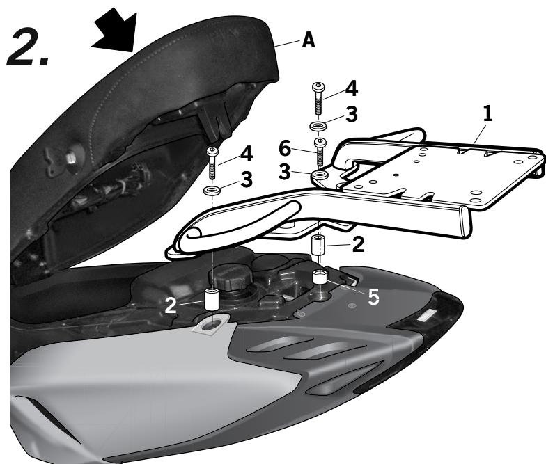
Set the spacers (2) and (5). Assemble the KIT TOP support (1), fix it in the front area by means of screws (4) and washers (3). And in the rear area by means of screws (6) and washers (3). Close the seat (A).
