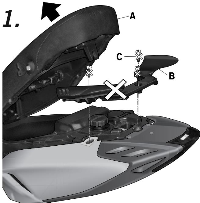
Dismantle the seat (A). Dismantle and remove handgrip (B) and the screws (C).
