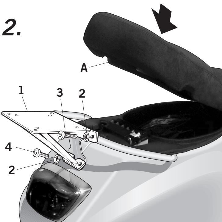
Assemble the KIT TOP support (1) in top area using the washers (2) and the screws (3). And in low area using the washers (2) and the screws (4).
