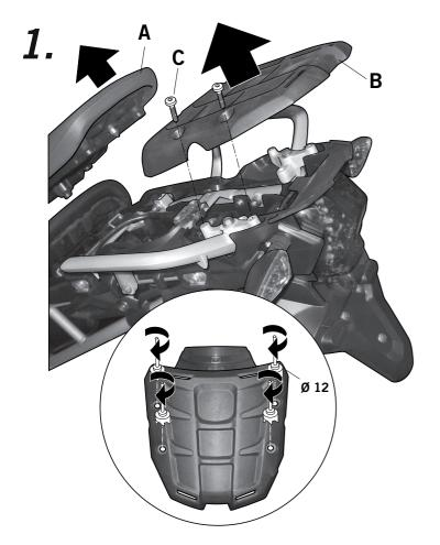
Dismantle the seat (A). Dismantle the embellishment cover (B) of the original rear luggage carrier, using the screws (C). Enlarge the four holes of the cover (B) to Ø12. Place the cover (B) over the original luggage carrier. Assemble the seat (A).
