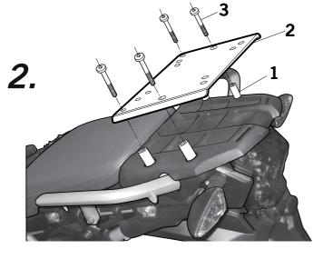
Assemble the spacers (1). Assemble the KIT TOP (2) and fasten it using the screws (3).
