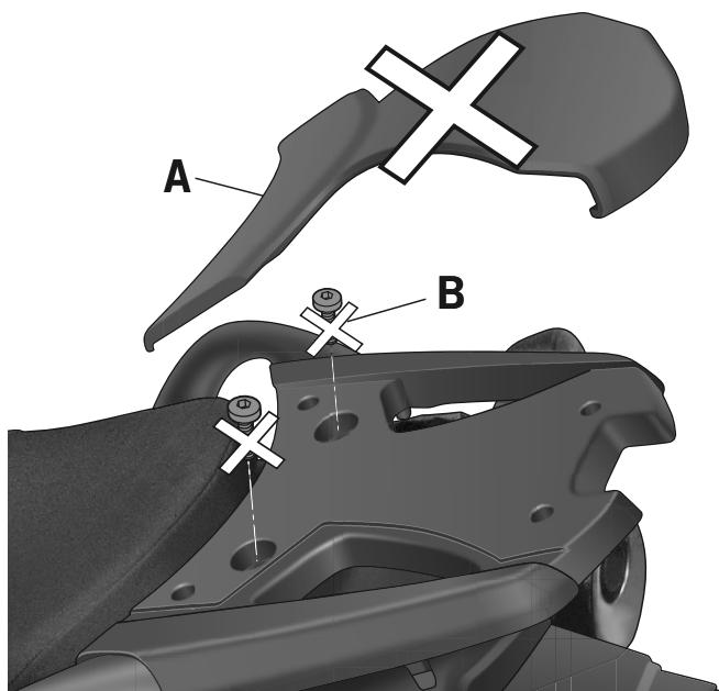
**Advice for correct fitting of the kit:** Do not fully tighten the screws until it is ensured that the KIT is correctly attached and aligned.
