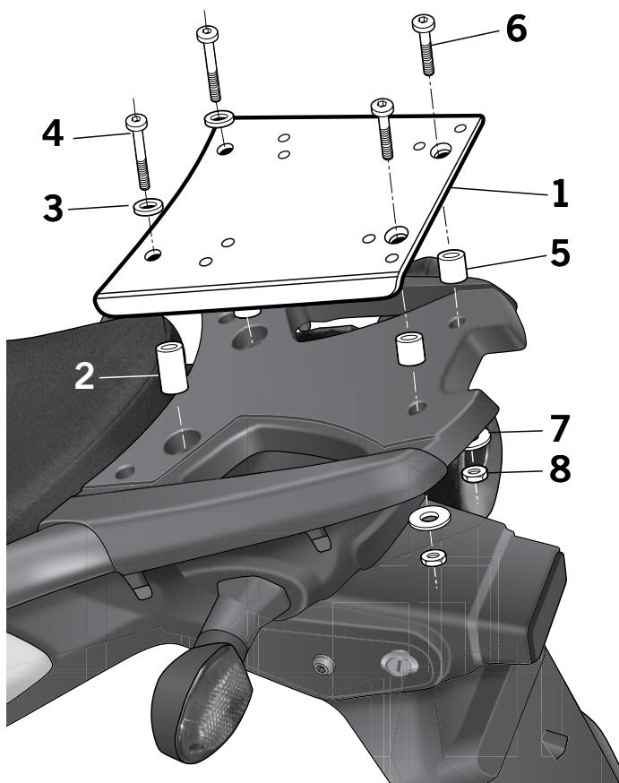
Assembly the KIT TOP support (1) in the frontal area by way of the lengthy spacers (2), the washers (3) and the screws (4), and in the rear area by means of the short spacers (5), the screws (6), the washers (7) and the nuts (8).
