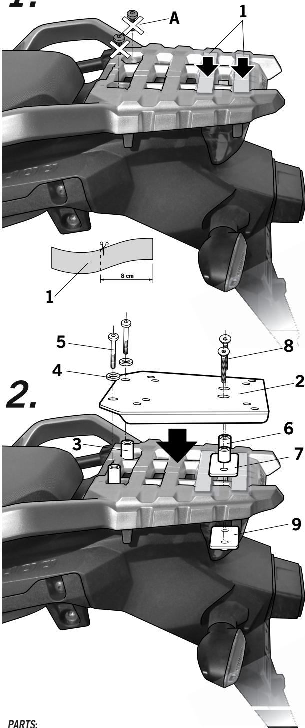
Disassembly and remove the screws (A) of the original rear rack. Replace them with the foam adhesives (1).
