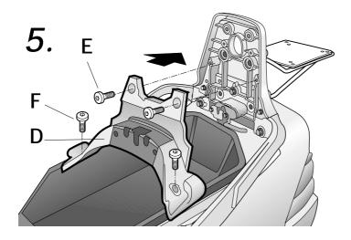
Mount the back hubcap (D) with the screws (E) and the screws (F).
