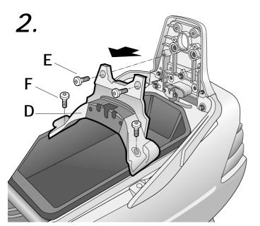
Remove the back hubcap (D) with the screws (E) and the screws (F).
