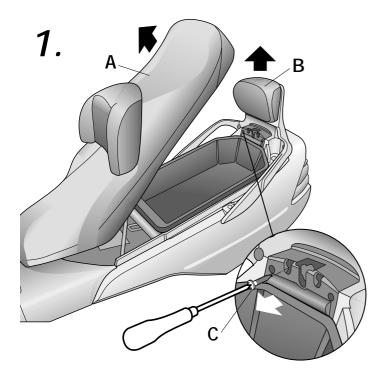
Open the seat (A). Remove the back cushion (B), with the interior screw (C). Note: use a screwdriver with a magnetised point, to facilitate the job.
