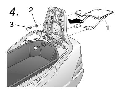
Mount kit top (1), on the back support, with the washers (2) and the screws (3).
