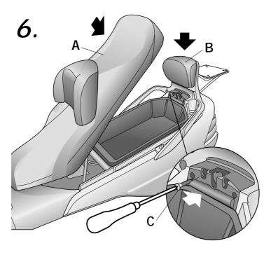
Mount the back cushion (B) with the screws (C). Note: Use the magnetised screwdriver again.
