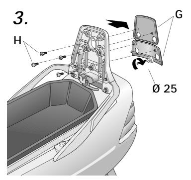
Remove the small back caps (G) with the screws (H). Make the holes Ø25 in the interior marks of the small lids, and once they have holes, mount them once again with the screws (H).
