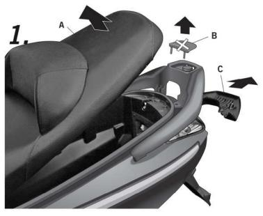
Open the seat (A). Dismantle the embellishment upper cap from the folding seat (B), which is discarded, and the lower cap (C).
