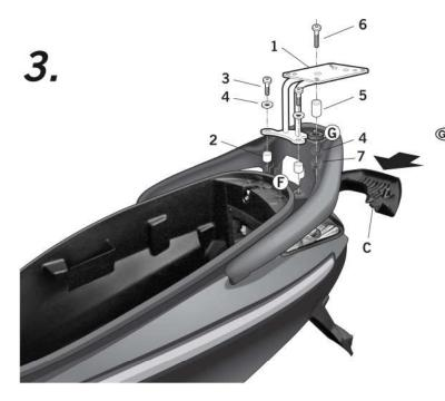
Assemble the KIT TOP upper support (1) in zone (F), with spacers (2), screws (3) and washers (4). And in zone (G), with the spacer (5), washer (4), screw (6) and nut (7). Assemble the bottom cap (C).
