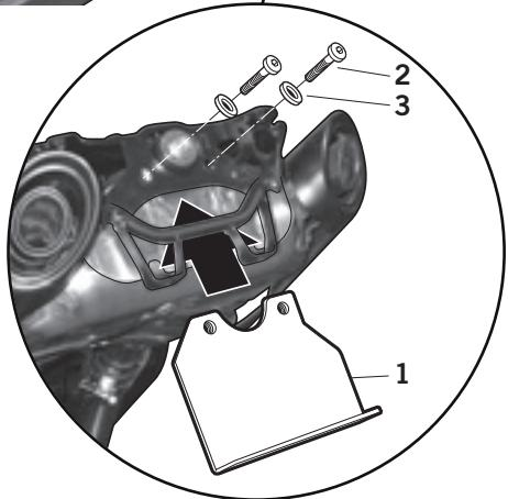
Follow the drawing to assemble the reinforcement support (1) in the chassis zone by means of the screws (2) and the washers (3).
