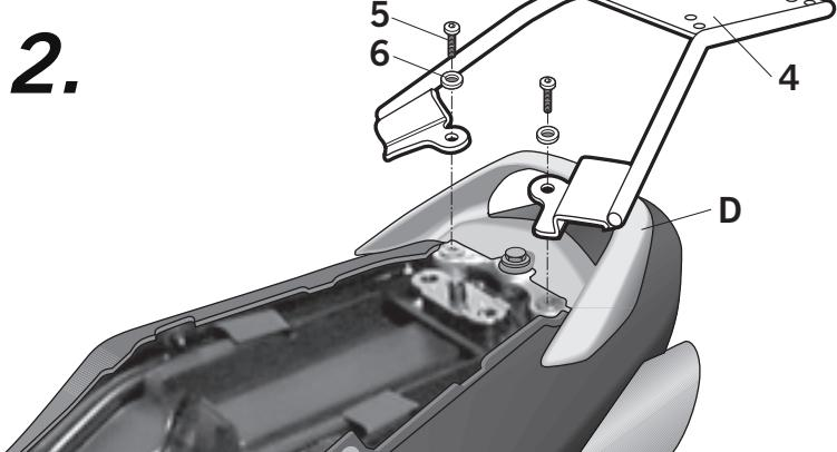
Assemble the KIT TOP support (4) over the handle (D), using the screws (5) and washers (6).
