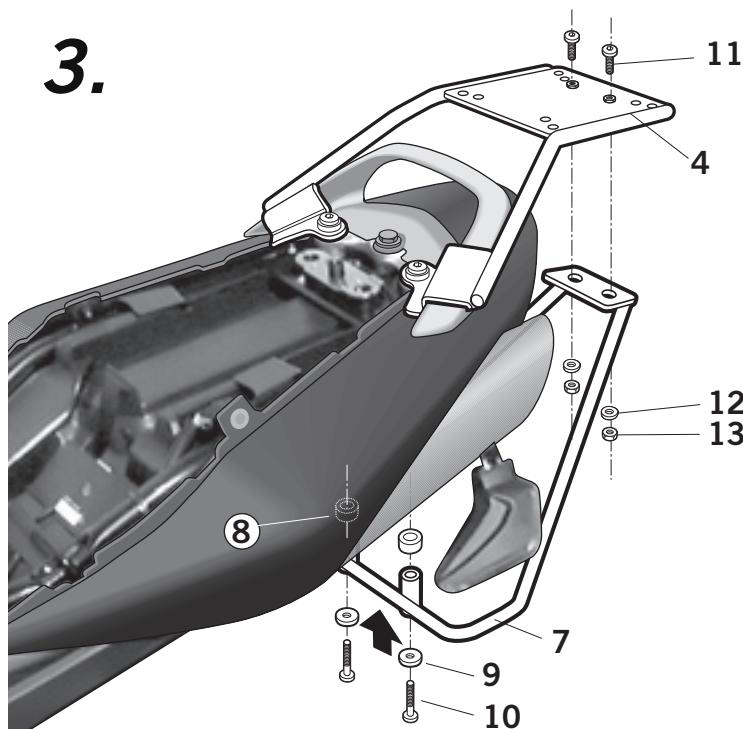
Assemble the KIT TOP union (7) with the spacers (8), the washers (9) and the screws (10).
