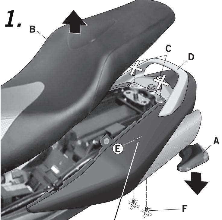
Dismantle the back indicators (A). Dismantle the seat (B). Dismantle and remove the lateral screws (C) from the handle (D) and in zone (E) underneath the fenders, the screws(F).
