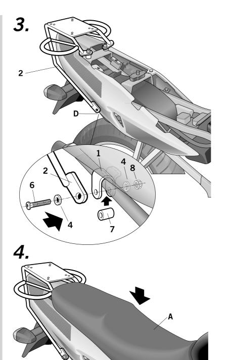
And in the chassis tube area using bridles (1), screws (6), washers (4), spacers (7) and
