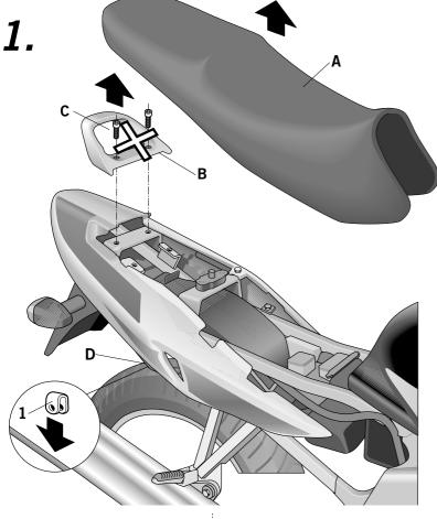
Dismantle seat (A). Dismantle and remove handgrip (B) using and removing screws (C). Attach bridles (1) onto the chassis tube, side
