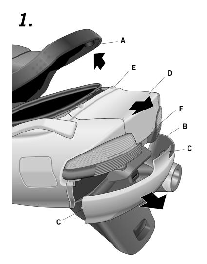
Make three holes  $\emptyset$ 17 in the indicated points of the inner side of the upper back body (D).
