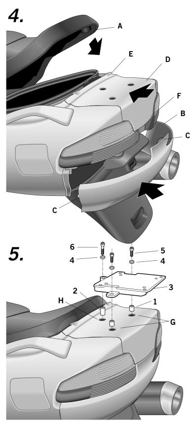
Assemble the lower (B) and the upper (D) back body parts, by means of the clips (C - E - F). (Note: execute carefully the disassembly of the body parts to avoid possible breaks). Close the seat (A).
