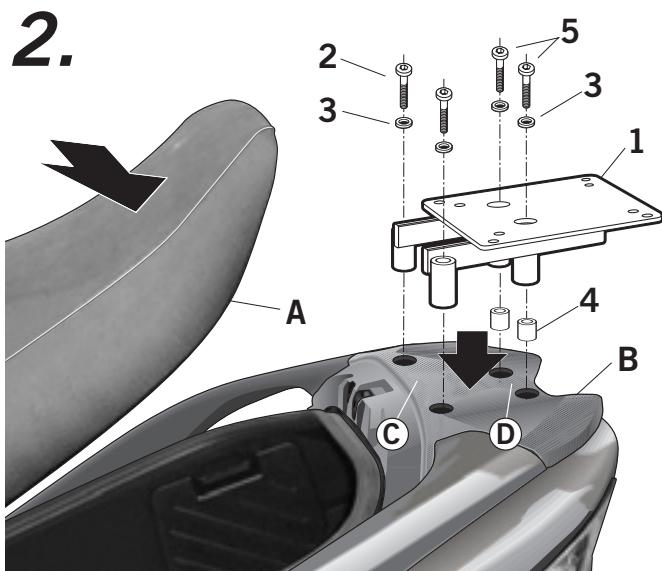
Re-assemble the back cover (B). Assemble the KIT TOP (1) support in the zone (C) using the screws (2) and the washers (3); and in the zone (D) using the spacers (4), the screws (5) and the washers (3). Close the seat (A).
