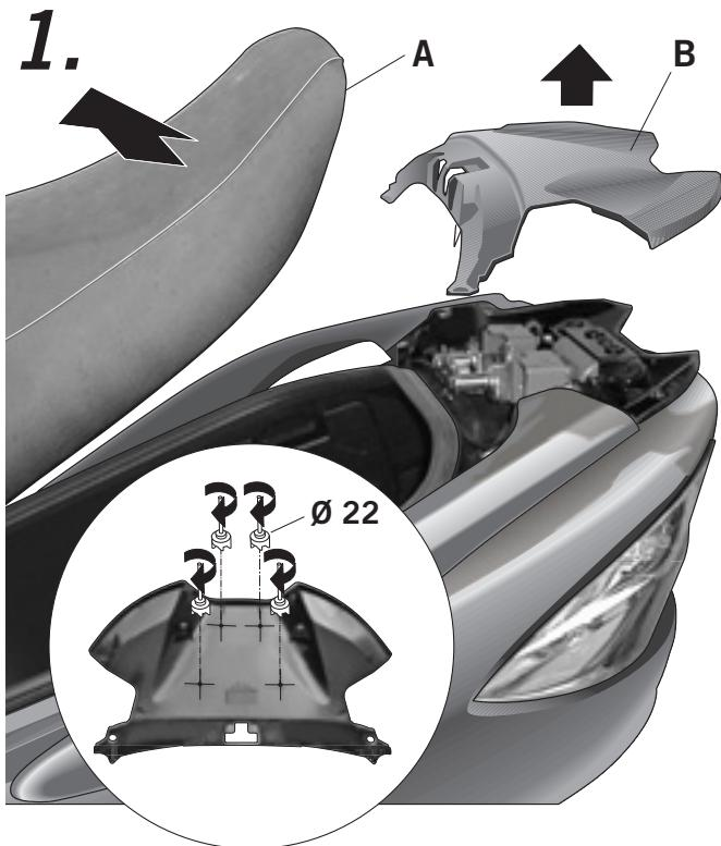
Open the seat (A). Disassemble the back cover (B).
