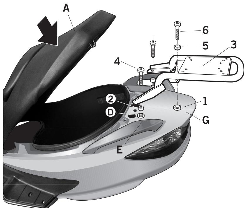
Assemble the KIT TOP carrier (3) in the (E) area, using the washers (D), the spacers (2) and the screws (4).
