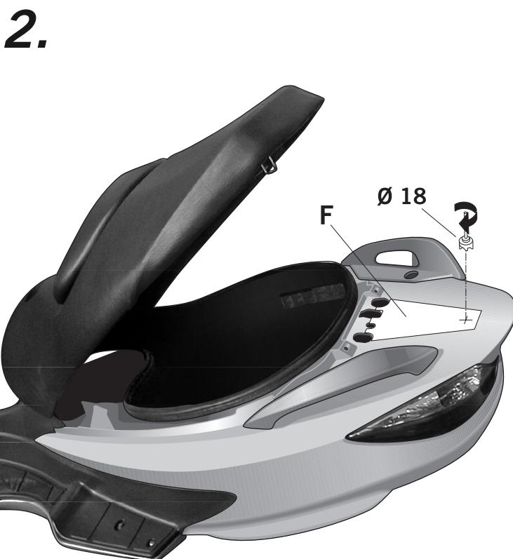
Cut out the pattern (F) included in the kit, placed it as shown in the picture, mark the center point and carry out a Ø18 mm hole (Note: It is recommended to make various holes of Ø inferior size until reaching a 18 mm diameter. The holing process will be carried out carefully in order to avoid the drill bits from touching the subchassis).
