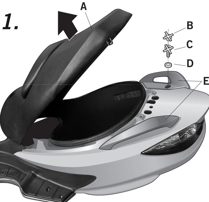
Open the seat (A). Dismantle the rear rubber stoppers (B), the rear screws (C) and the washers (D) of the lateral grips (E) (Note: discard the stoppers (B) and screws (C)).
