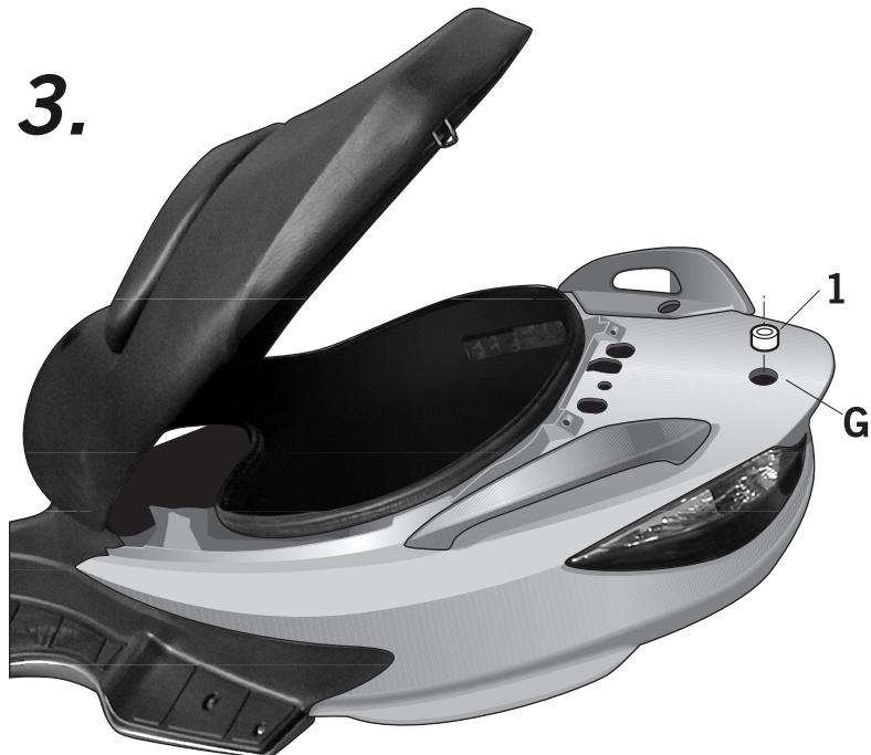
Place the spacer (1) in the Ø18 hole, (G) area.
