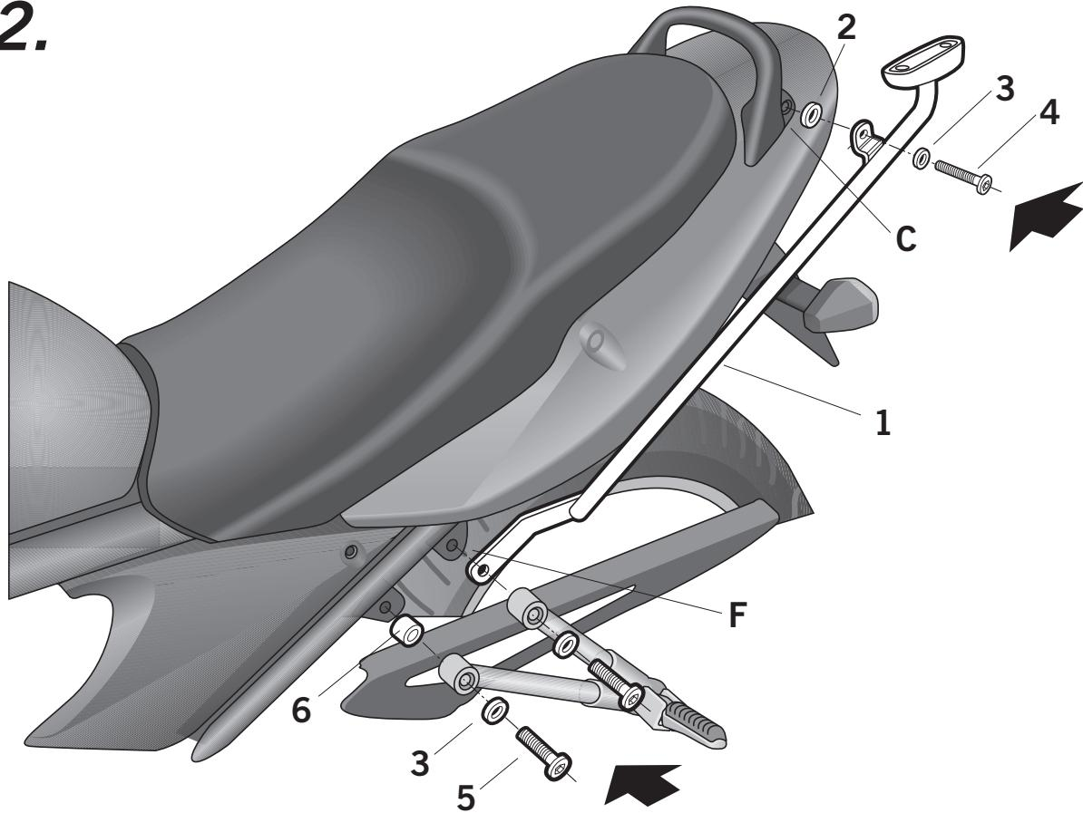
Assemble the KIT TOP support(1) in area (C), using the distance pieces (2), the washers (3) and the screws (4).
