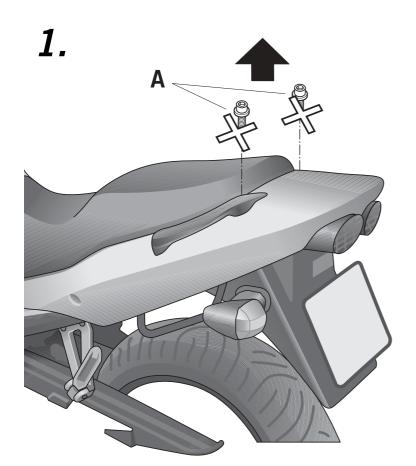
Advice for correct fitting of the kit: Do not fully tighten the screws until sure that the kit is correctly positioned and aligned. Note: If the bike already has full kit (KOZR79SF) assemble kit top (KOZR71ST) according to the instructions and remove spacers(1).
