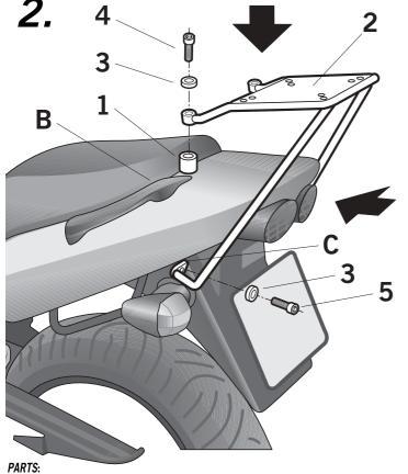
Position spacers (1) in the side handgrips. Assemble the kit top support (2) using washers (3) and screws (4) in area (B) of the handgrip, and in area (C) orf the chassis using washers (3) and screws (5).
