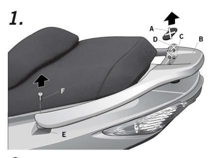
(A) of the back handle (B). Dismantle and put aside in area (C) the screws (D) and loosen in area (E) the screws (F).
