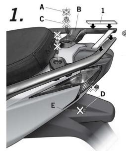
(B) Disassembly and remove plastic covers (A) from the rear handle (B) as well as the screws (C) that must be removed too. Disassembly and remove the screws (D) from the rear mudguard, area (E). Put the foam layer (1) in the original luggage rack, so as to protect the contact area.
