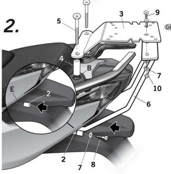
**(B)** Place the threaded spacers M6 (2) in the area (E). Assembly the KIT TOPMASTER (3) to the rear handle (B), using the spacers (4) and the screws (5). And in the area (E), by means of threaded spacers M6 (2), washers (7) and screws (8). Assemble the KIT TOP (3) together with rib support (6), by means of the screws (9), the washers (7) and the nuts (10).
