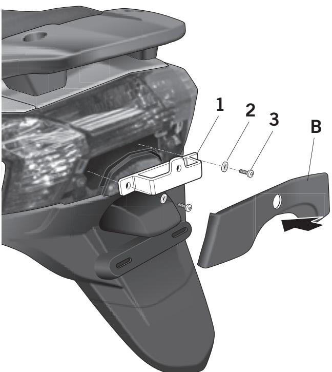
In the interior zone, lace the Top union piece (1) by means of the washers (2) and the screws(3). Assemble the embellishment cover (B).
