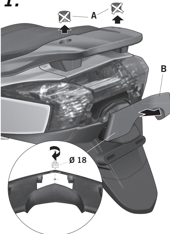
Disassemble and discard the cover (A) of the motorcycle's original luggage carrier. Disassemble the motorcycle's rear fairing (B). This operation must be done with extreme care since the fairing is fastened by plastic clips. Next, cut the stencil included in this kit and place it according to the drawing. Make two marks and drill two  $18 \varnothing$  holes. (Note: we suggest making first lower  $\varnothing$  holes until reaching a  $\varnothing$  of 18 mm).
