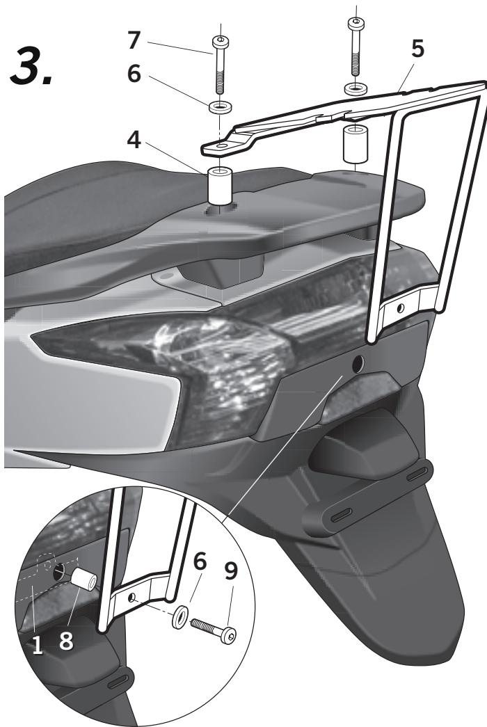
Place the spacers (4), and assemble the KIT TOP (5) over the original luggage carried by means of the spacers (4), washers (6) and screws (7). Fasten it to the Top union piece (1) by means of the spacer (8), the washer (6) and the screw (9).
