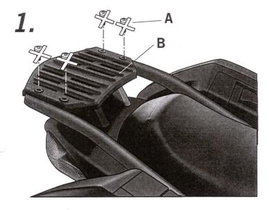
**GB** Disassemble and discard the screws (A) from the rack (B). Leave the original spacers in their place.
