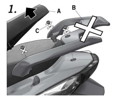
GB Open the rear seat (A), disassemble and remove the original handrail (B) and the screws (C).
