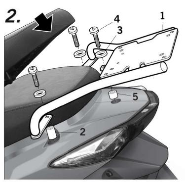
**GB** Place the KIT TOP (1) support, by means of the spacers (2), the washers (3) and the nuts (4), and in the rear area by means of the spacer (5), the washer (3) and the nut (4). Close the seat (A).
