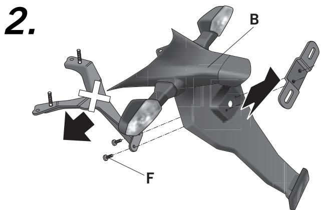
Disassemble and discard the reinforcement support (F) form the back mudguard (B).
