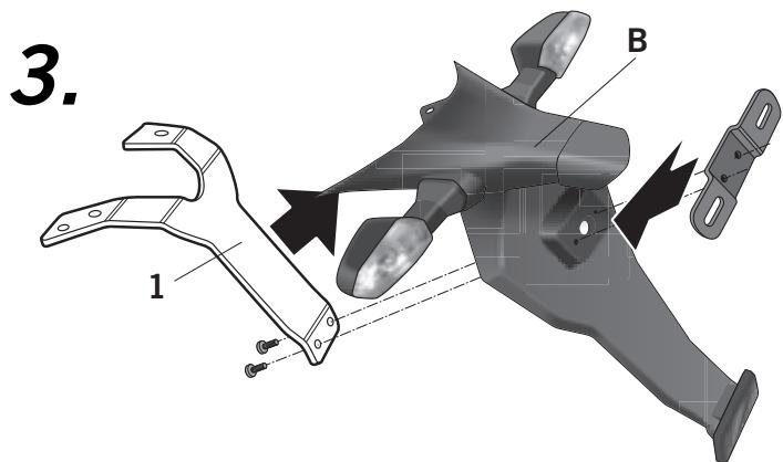
Assemble this Kit's reinforcement support (1) to the back mudguard (B).
