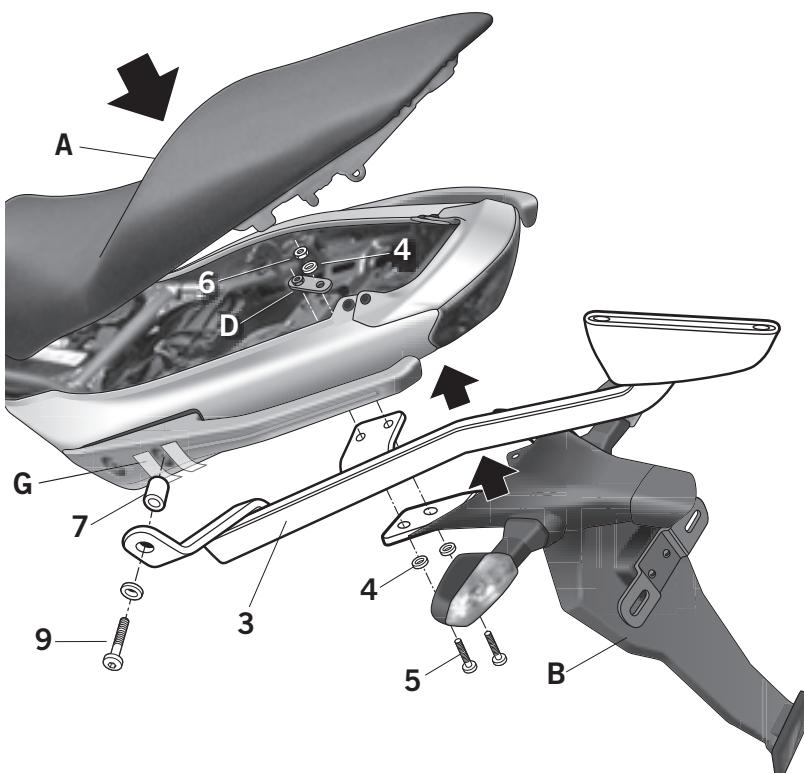
Place the KIT TOP supports (3) between the lower part of the motorcycle and the rear mudguard (B), by means of the washers (4) and the screws (5) in the lower zone, and by means of the interior plates (D), the nuts (6) and the washers (4) in the upper zone. And in zone (G), by means of the spacers (7), the washers (8) and the screws (9). Assemble the seat (A).
