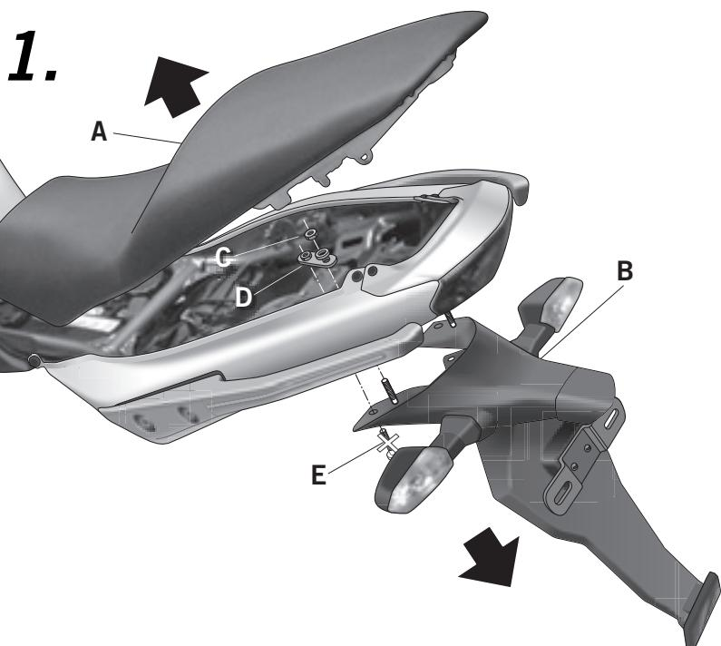
Disassemble the seat(A). Disassemble the rear mudguard (B) by means of the interior nuts (C) and inferior screws (E) which must be discarded. Note: do not discard the interior plates (D) since they will be used during the assembly process.
